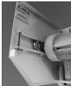
The rolling bracket ensures smooth operation and reduces wear.
